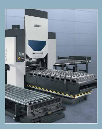
Dirt and material residues can accumulate in the leveling unit during daily production. Thorough cleaning of the leveling rollers and back-up rollers provides consistent leveling results and prevents damage due to contamination of the leveling unit. For this reason, the FlatMaster® is fitted with a quick change of the leveling rollers. The leveling rollers can be changed, and the unit thoroughly cleaned, in minutes.
