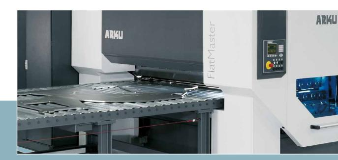
In roller leveling, a sheet metal part is deformed by a series of alternate bends so that in the end it is flat and nearly stress-free. The smaller the residual stress in the flame-cut parts, the better the results in subsequent welding, bending or chamfering processes.
